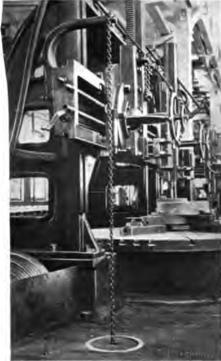
Fig. 1. Counterweight suspended underneath Floor.*
